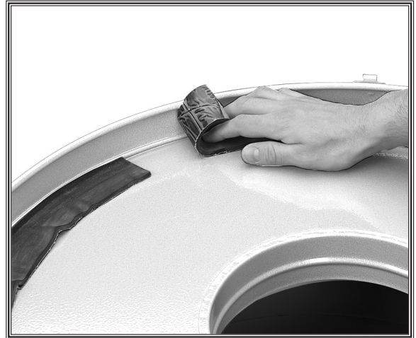
Figure 29. Attaching foam tape to collector drum lid.
